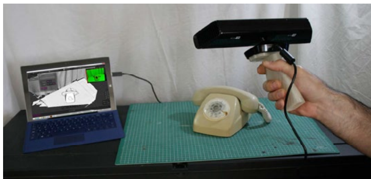
Fig. 1. Scanning process using Kinect Xbox 360 (left) and software Skanect Pro (right)
