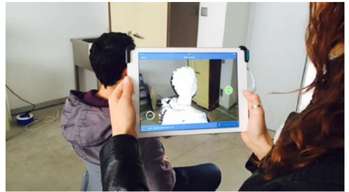
Fig. 2 Scanning process using Structure Sensor for iPad and software ItSeez3D
