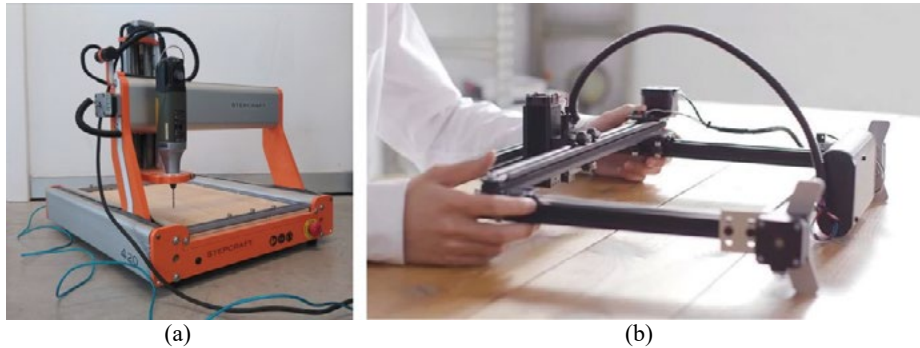
Figure 2a: Hobby-oriented milling machine: Stepcraft 420
