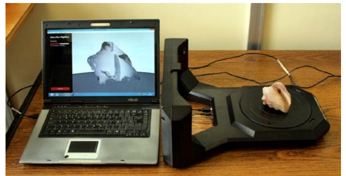
Fig. 4. Scanning process of a fossil using MakerBot Digitizer
